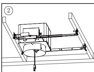
2. Repeat step 1, put the construction can on another side fix the brackets with nails.
