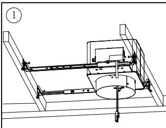
1. Put the construction can on one side and fix the brackets with nails.
