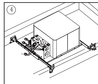
4. Knock out the knock hole and assemble the flexible metal conduit. Open the junction box, and connect the house wire accurately according to the instruction. The black wire connects to the fire wire, the white wire connects to the middle wire, and the ground wire connects to the green wire.
