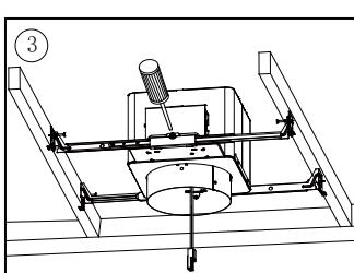
3. Move the construction can to the proper location and screw it.
