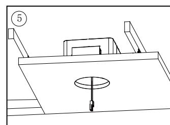
5. Assembly the ceiling and use the template hole to dig out an installation hole in the installation location. Finally connect the fixture to be installed with the construction can. You can use lighting housing smoothly!
