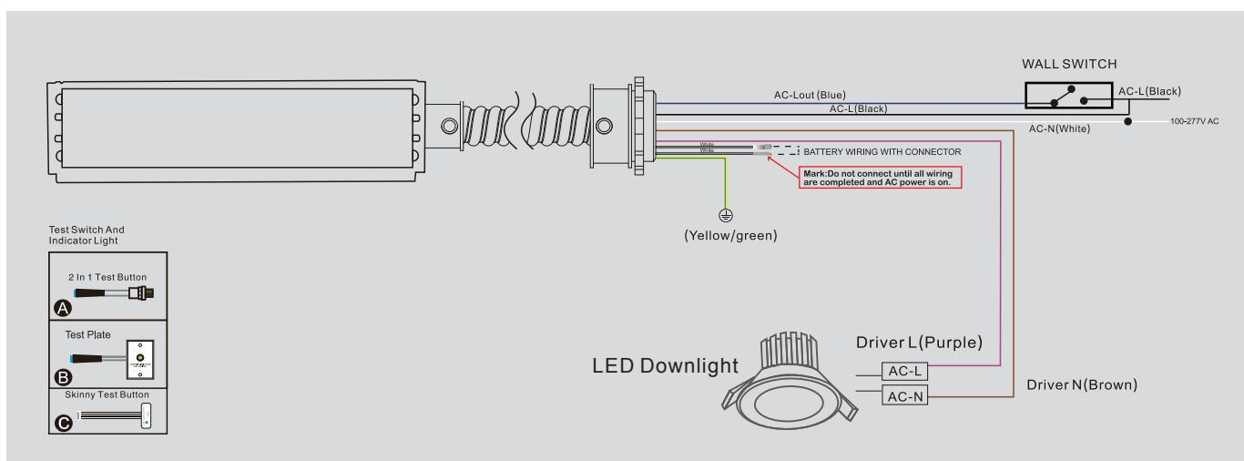
Emergency Driver can be used with either a switched or unswitched or emergency only fixture. If a switched fixture is used, an unswitched hot lead must be connected to the emergency driver.
