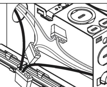
3. Remove the mounting clips from the housing can. Place the housing can onto the ceiling through the pre-cutting hole.
