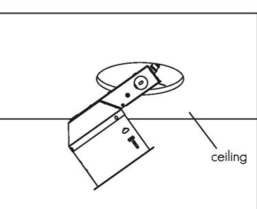
4. Install all the mounting clips back to the housing can. Push the mounting clips through the T-socket until they snap onto the ceiling. Secure the housing can to complete the installation.
